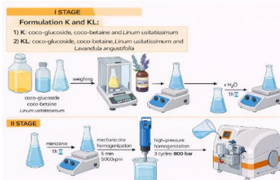
Figure 1. A scheme for obtaining emulsions and selecting formulation components.
